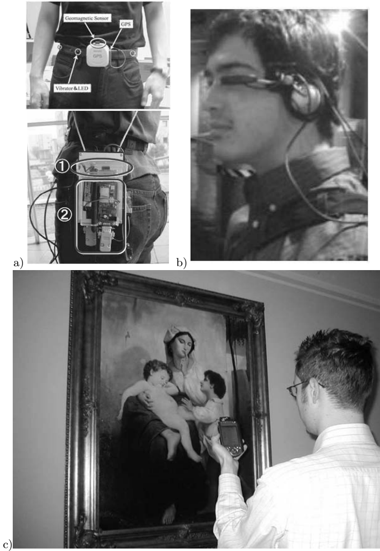
Fig. 2.2. The medium scale: wearable and handheld computing devices. (a) A belt wearable computing infrastructure; image taken from [149]; (b) Head-up wearable display; image taken from [134]; (c) A tourist accessing information on site by a PDA
